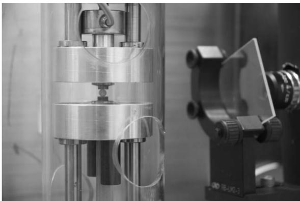
Figure 2. Photograph of specimen in *in situ* load frame in x-ray beamline. Phosphor scintillator and microscope lens are visible to the right of frame.
