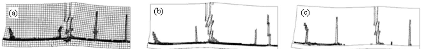
Figure 7. Crack patterns of the concrete wall with no reinforcement, in the case of perfect bond between wall and foundation (a), and rough (b) or smooth (c) interface.
