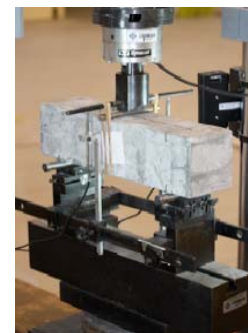
Figure 1. Test for fracture energy.
