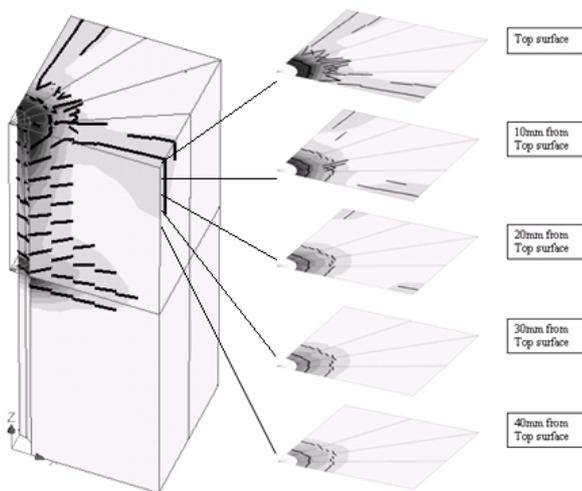
Figure 10. Crack width plot and crack pattern at peak load of I-model.
