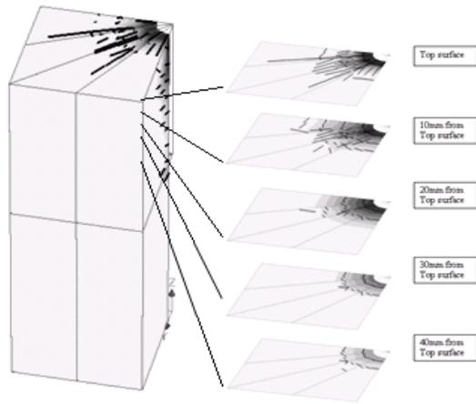
Figure 6. Crack width plot and crack pattern at peak load of HSCC DTP-BT-50N/m model.
