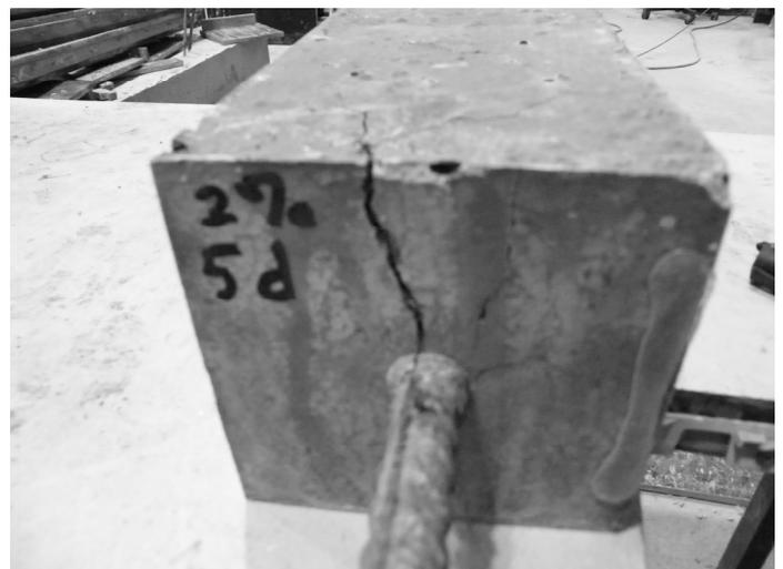
Figure 8. Tensile splitting failure of HSFRC under DTP-BT.
