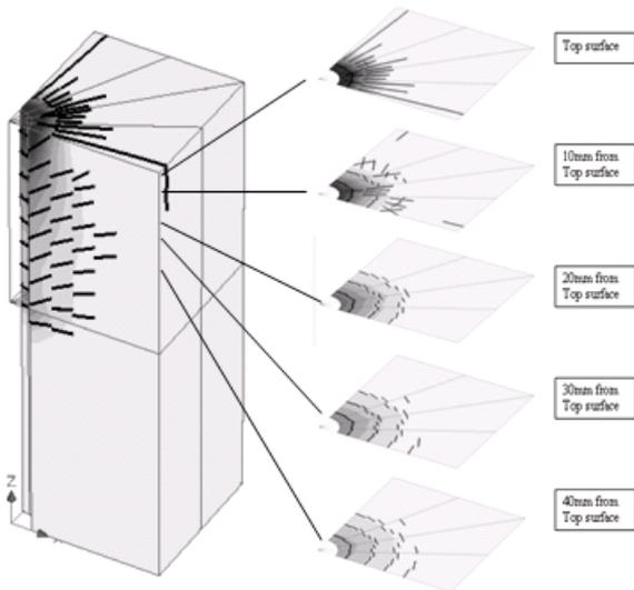
Figure 9. Crack width plot and crack pattern at peak load of H-model.
