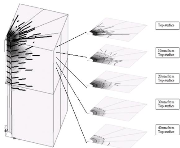
Figure 5. Crack width plot and crack pattern at peak load of HSCC DTP-BT-75N/m model.
