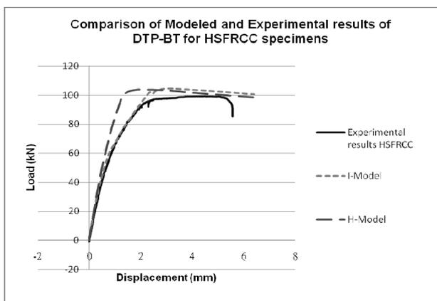
Figure 7. Load-displacement curves of H-model, I-model and experimental results.
