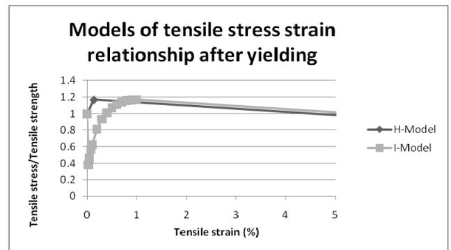
Figure 3. Tensile stress strain relationships of H-Model and I-Model.
