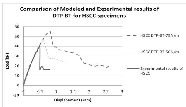
Figure 4. Load-displacement curves of HSCC models and experimental results.
