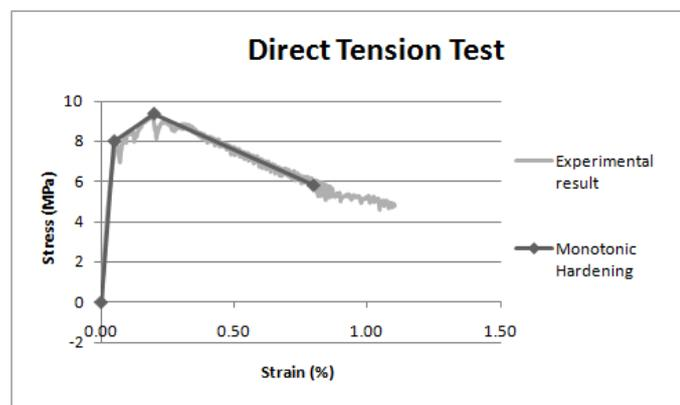
Figure 1. Tensile stress strain curve of HSFRC and monotonic hardening model.
