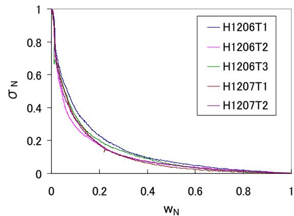
Figure 8. Tension softening curves (Mix B3).
