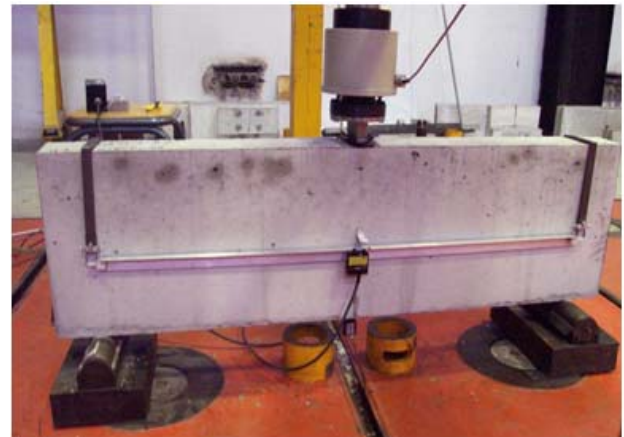
Figure 1. General view of experimental fracture test setup.
