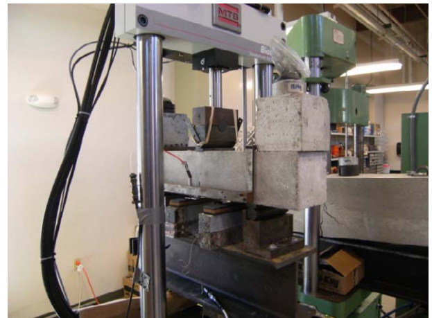
Figure 4. Notched beam level II (NB-LII) test set-up to extract cohesive fracture parameters.
