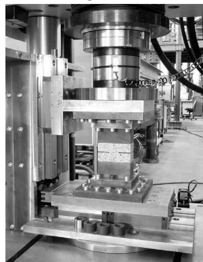
Figure 3. Test set-up showing a glued in test specimen, vertical load cell, support structure and the slides in both vertical and horizontal direction.
