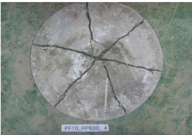
Figure 12. Crack pattern-2 of ring supported panel.
