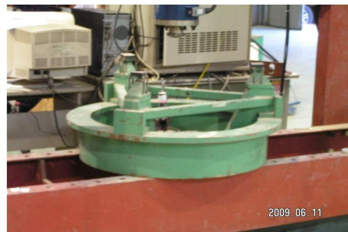
Figure 6. Apparatus for the point supported panel.
