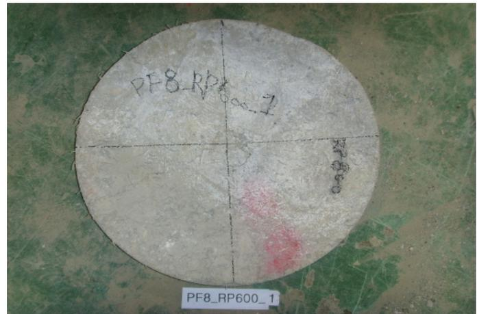
Figure 8. The ring supported panel specimen.
