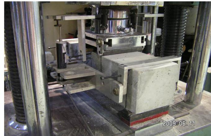
Figure 5. Toughness test of beam specimen.
