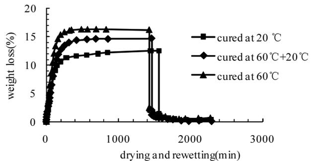
Figure 4. Weight loss of normal, heat treated and heat cured cement pastes with drying and rewetting time when dried at 43%RH and subsequently rewetted.
