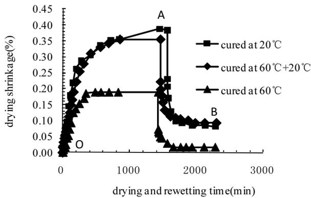
Figure 2. Drying shrinkage of normal, heat treated and heat cured cement pastes with drying and rewetting time when dried at 43%RH and subsequently rewetted.
