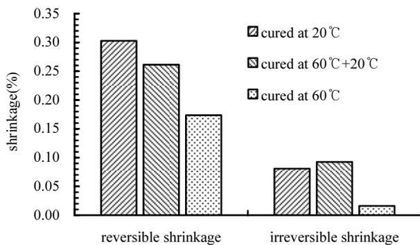
Figure 3. Reversible and irreversible drying shrinkage of normal, heat treated and heat cured cement pastes when dried at 43%RH.
