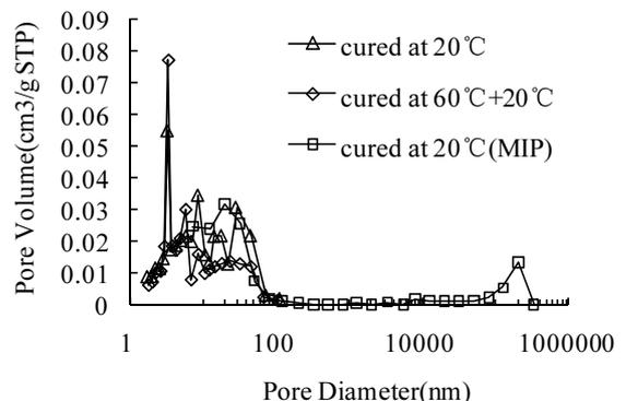
Figure 5. Pore size distribution of cement pastes with different curing regime, measured by nitrogen adsorption and desorption (Note: "cured at 20°C (MIP)" referred the the pore size distribution of the cement paste cured at 20 °C which was measured by Mercury Intrusion Porosimetry (MIP), as a reference only).
