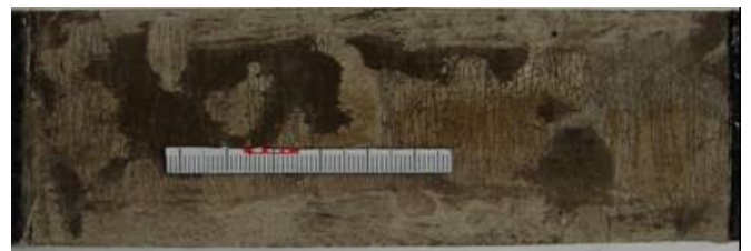
Figure 2. Crack pattern of UHTCC under tensile loading.
