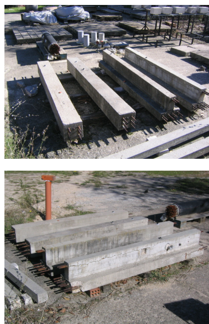
Figure 2. Exposition of elements to the atmosphere.
