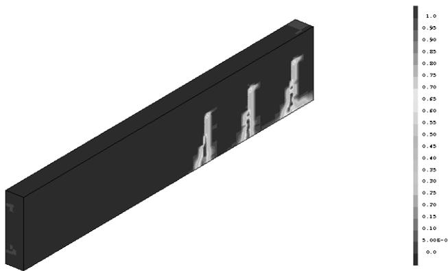
Figure 10. Cracks pattern after 25 years, under cyclic environmental conditions.
