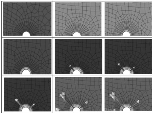
Figure 3. Evolution of the cracks pattern with time. Top: 3 cm concrete cover, bottom: 6 cm concrete cover.
