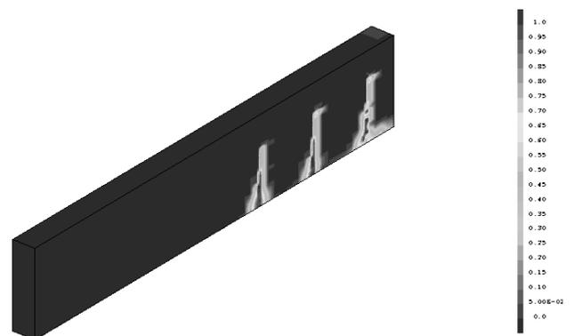
Figure 5. Cracks pattern under 3 points bending load.
