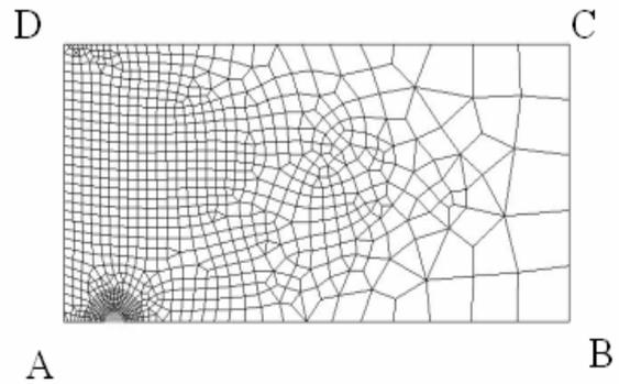
Figure 2. Mesh of the half slab (symmetry axis along AB).
