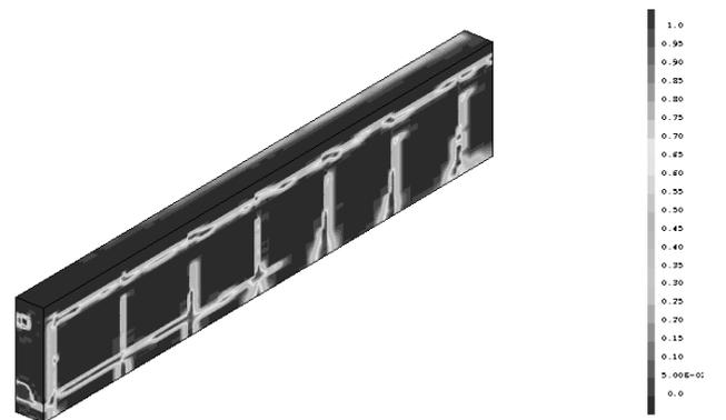
Figure 9. Cracks pattern after 50 years.
