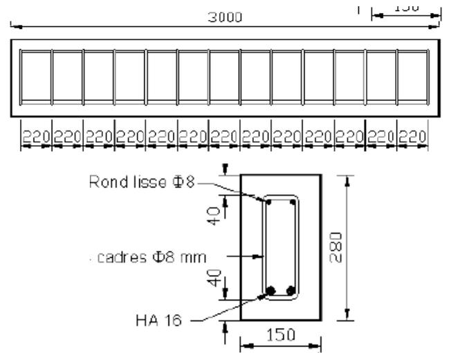
Figure 4. Beam dimensions and reinforcements.
