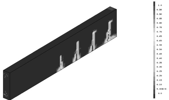
Figure 8. Cracks pattern after 25 years.
