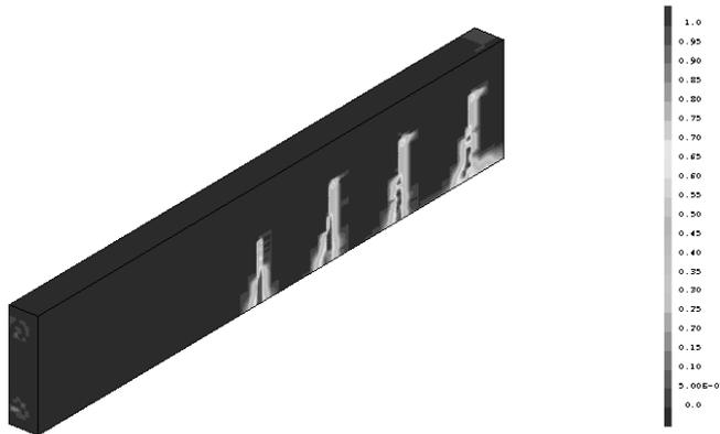
Figure 11. Cracks pattern after 50 years, under cyclic environmental conditions.
