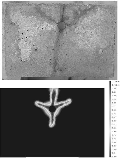
Figure 1. Comparison of cracks pattern, after 40 hours of accelerated corrosion, between experiment (top) and prediction (bottom).
