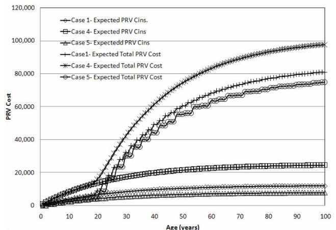
Figure 8. Effect of inspection interval period on life cycle cost.
