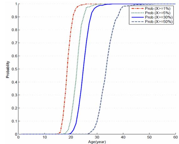
Figure 6. Probability of Exceeding of extent of cracked area from and acceptable threshold.
