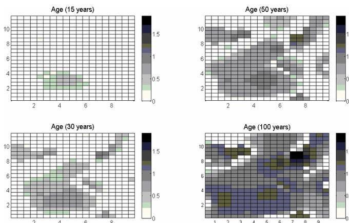
Figure 4. Random realization of spatial variation of crack width increase with time.
