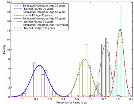
Figure 5. Distribution of extent of damaged area in different ages of service life of bridge deck.
