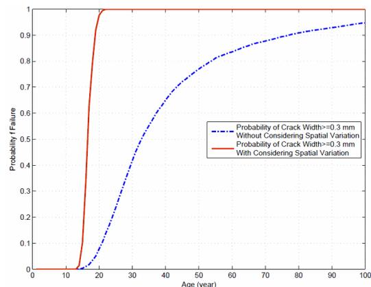
Figure 3. The effect of considering spatial variability on estimated probability of failure.
