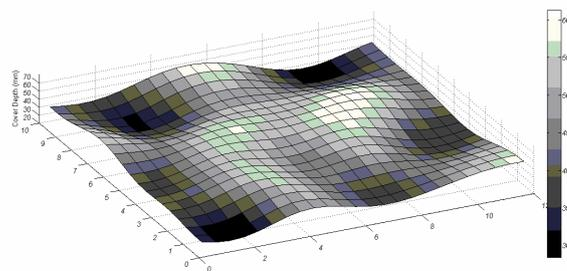
Figure 2. Random Realization of spatially variable cover depth of concrete deck.
