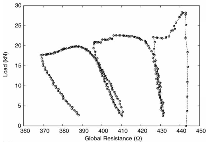
Figure 6. Load vs. global resistance.
