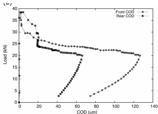
Figure 2. Load vs front and rear COD.
