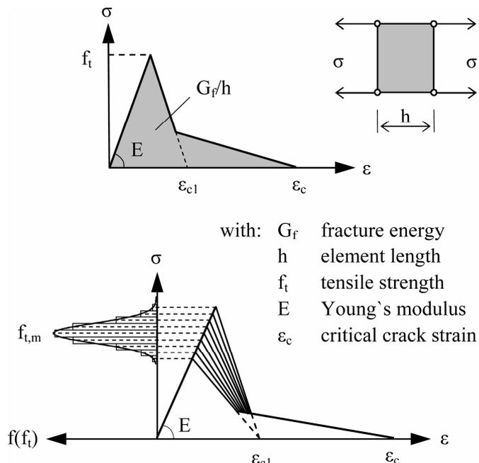
Figure 6. Implementation of the Crack Band Model in the finite element model (above) and consideration of the heterogeneity of the sandstone (below).
