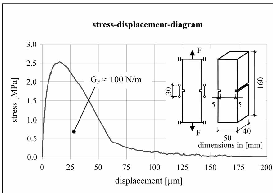
Figure 1. Experimental setup, characteristic curve progression and geometry of the notched samples.
