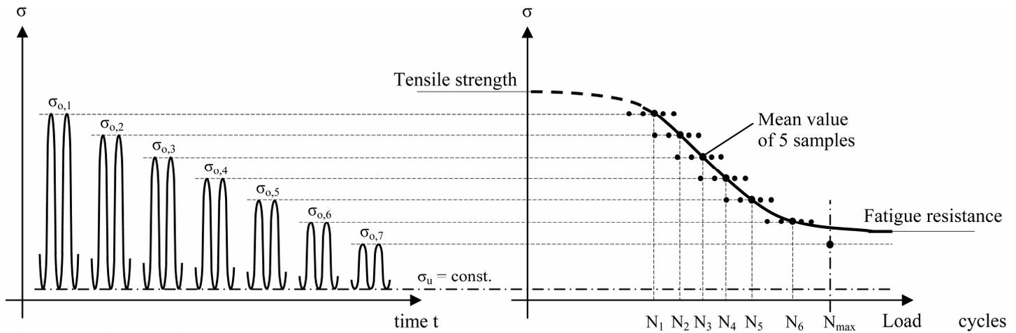
Figure 2. Evaluation of the Woehler curve with constant lower stress  $\sigma_u$ .
