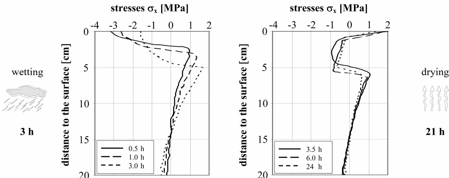
Figure 7. Self-equilibrating stresses due to hygral strain. Left diagram: during three hours of wetting. Right diagram: during 21 hours of drying.
