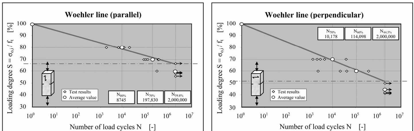
Figure 3. Test results of the dynamic tensile tests.
