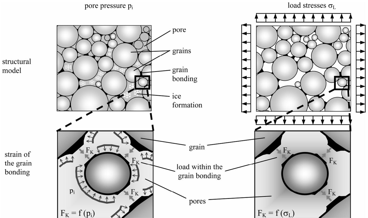
Figure 9. Exposure of the structural model to the effect of pore pressure due to ice formation (left) and load stresses (right).
