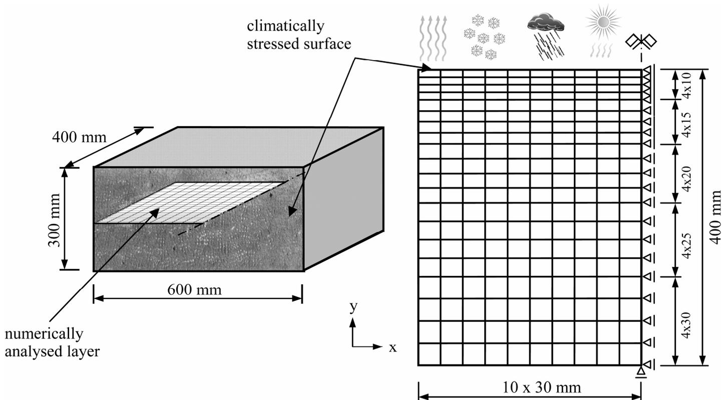
Figure 4. Numerically analysed layer of the sandstone continuum and discretised system.
