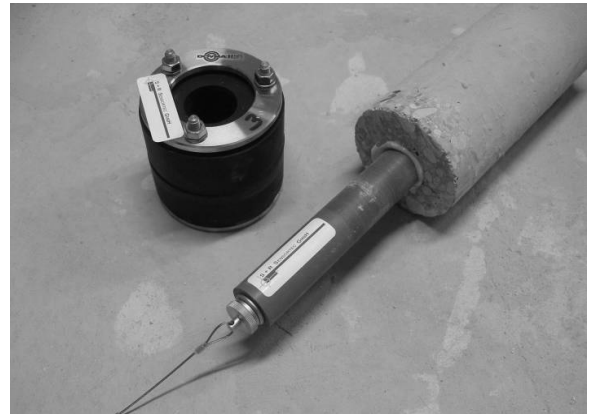
Figure 20. Acid sensors ready for installation: The figure shows the drilled concrete core, the multipolar plug and a sealing gasket to ensure density of the sensor installation.
