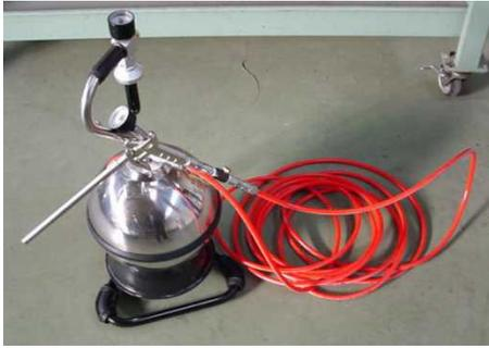
Figure 2. Portable compressor and a shooting device.
