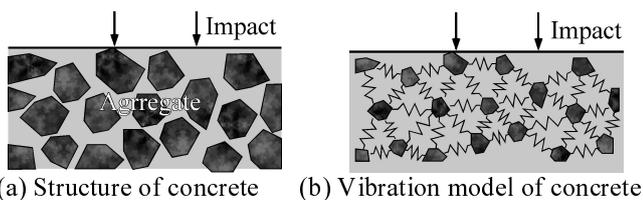
Figure 7. Structure of concrete and its vibration model.
