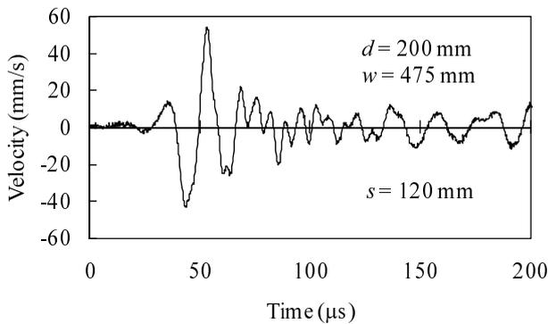
Figure 5. Surface velocity in time domain for one test.
