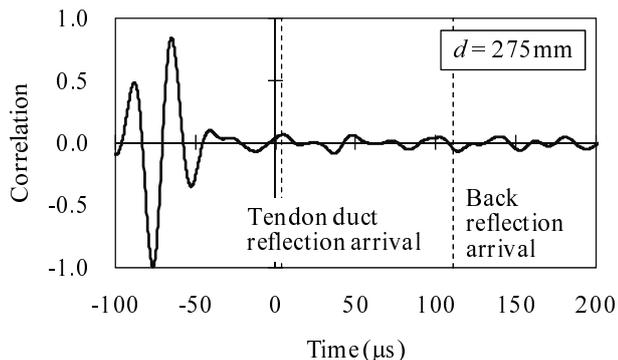
Figure 11. Correlation function for grouted tendon duct.
