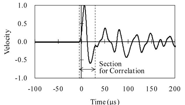
Figure 9. Velocity on back surface and section for correlation.
