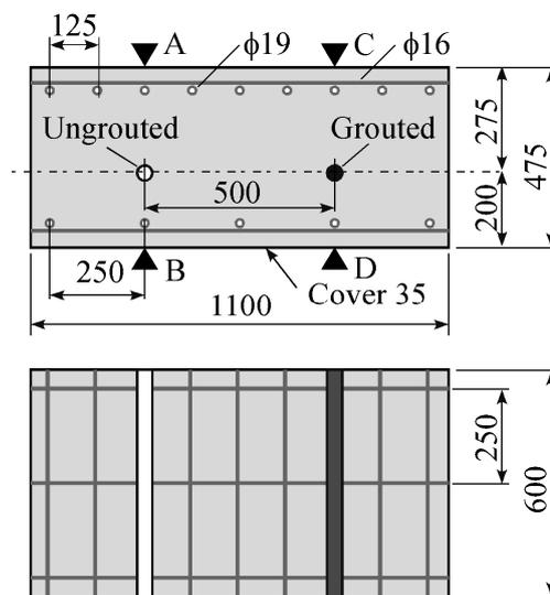
Figure 1. Specimen for impact echo tests.
