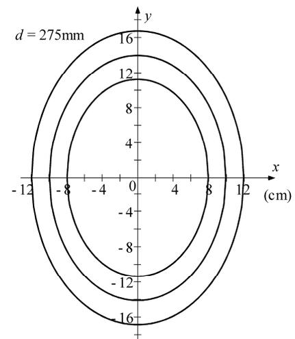
Figure 4. The impact points on the surface for the constant length of the elastic wave path.
