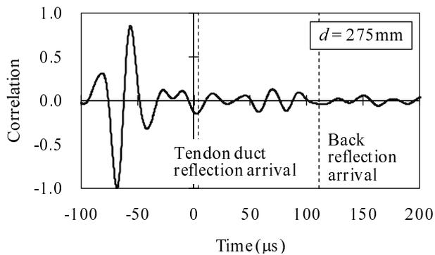
Figure 10. Correlation function for ungrouted tendon duct.
