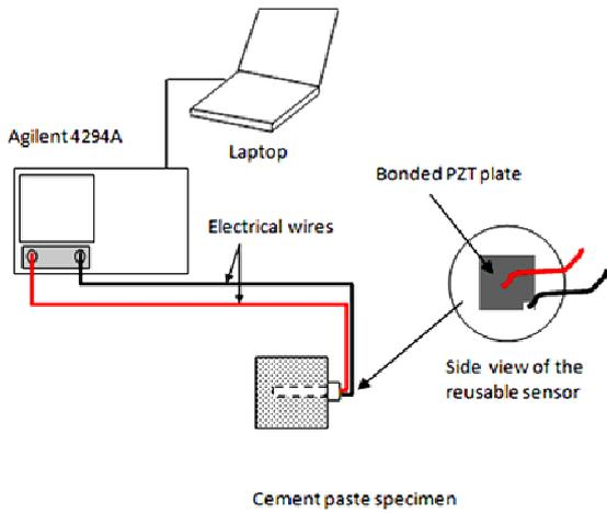
Figure 1. Schematic diagram of the monitoring system.
