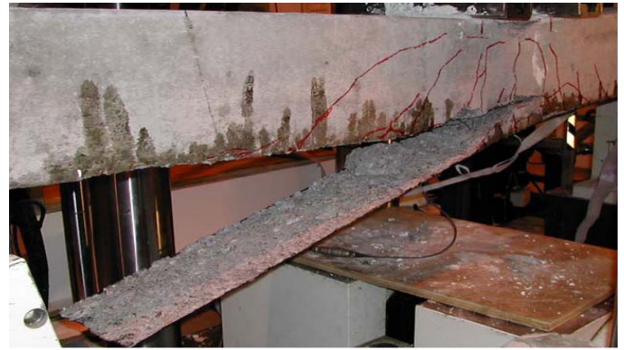
Figure 7. Intermediate crack induced debonding for the beam C5-M043-L6.
