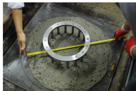
Figure 3. J-Ring test of fresh concrete.
