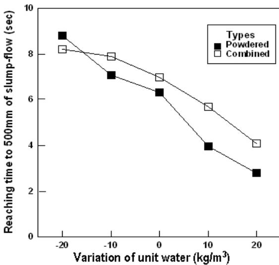
Figure 4. Reaching time to Slump-flow 500 mm.
