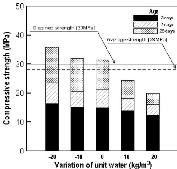
Figure 6. Compressive strength of the powdered high fluidity concrete.
