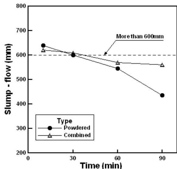
Figure 2. Slump-flow loss.
