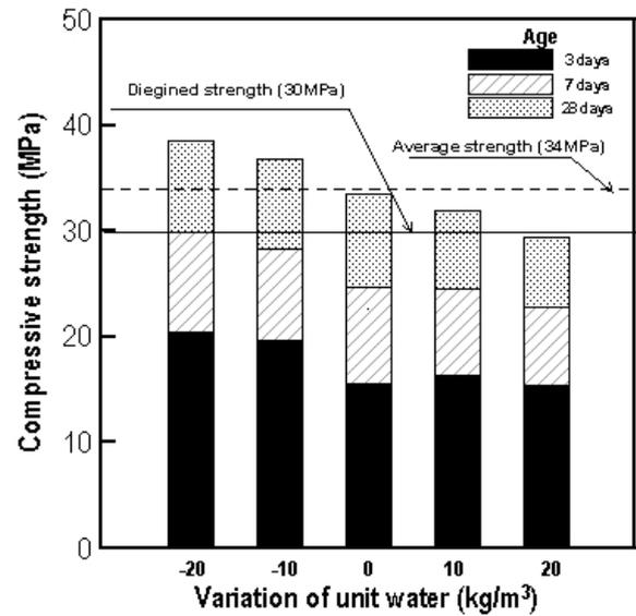
Figure 7. Compressive strength of the combined high fluidity concrete.
