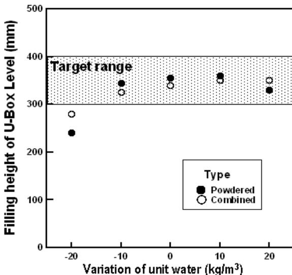
Figure 5. Filling height of U-Box.
