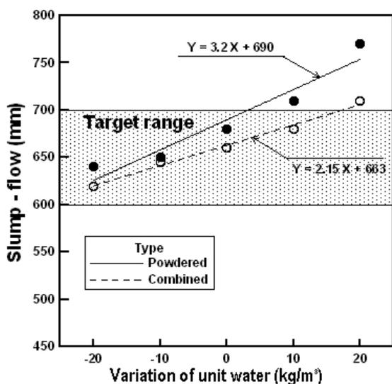
Figure 1. Slump-flow of high fluidity concrete.
