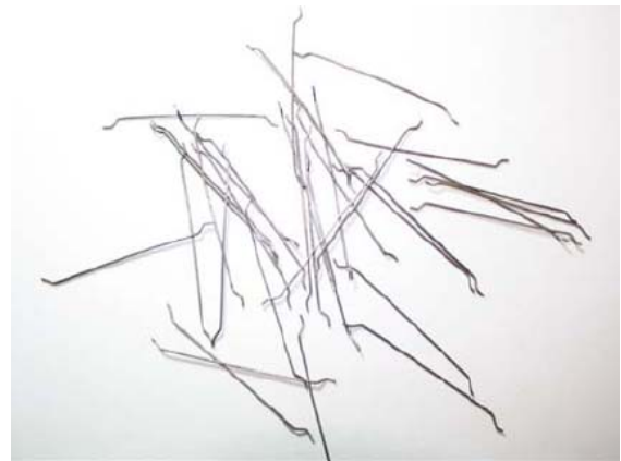
Figure 1. Discrete hooked steel fibers.
