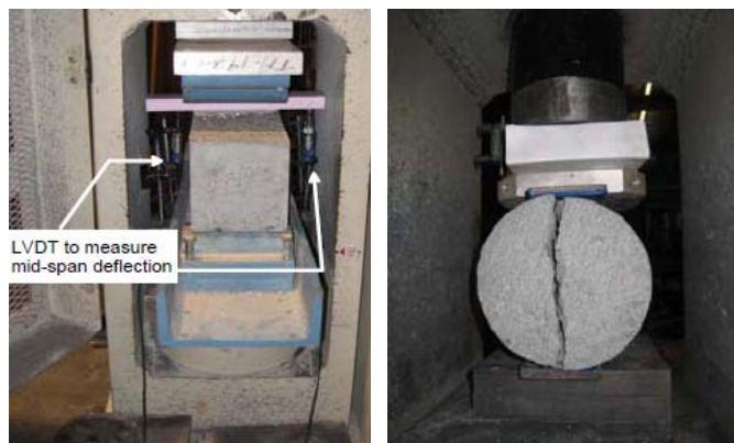
Figure 4. Modulus of rupture testing (per ASTM C1609) and splitting tensile strength testing (per ASTM C496) of concrete mixes (at Fears Lab of the University of Oklahoma).
