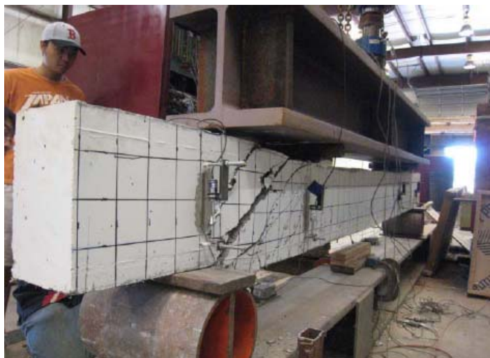
Figure 3. Four-point loading of a steel fiber-reinforced beam (at Fears Lab of the University of Oklahoma).
