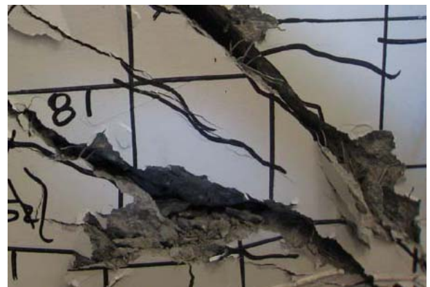
Figure 2. Steel fibers that restrain crack opening during shear testing (at Fears Lab of the University of Oklahoma).
