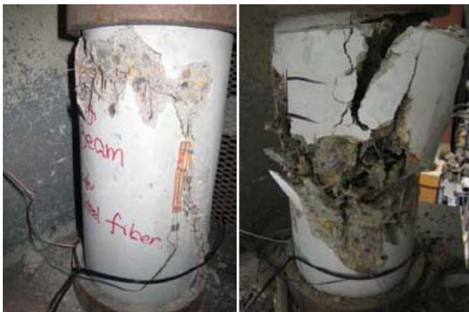
Figure 5. Compressive strength tests of SFRLC cylinders per ASTM C496, with two strain gauges per cylinder to measure strains (at Fears Lab of the University of Oklahoma). Note that red gravels exposed are expanded shale lightweight aggregates.
