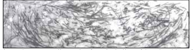
Figure 3. X-ray radiograph of vertical slice of SFRC subjected to superimposed orthogonal grid for counting intersections with fiber projections (Stroeven & Shah 1978). The results obtained showed the fiber structure to reveal partially linear planar orientation; the compaction by vibration-induced re-orientation in horizontal direction and the influence of the sides of the mould are obvious.
