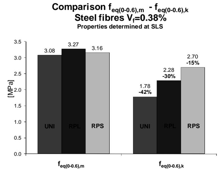
Figure 24. Average vs. characteristic  $f_{eq(0-0.6)}$  using the scatter of different standards: Round Panel tests vs. Beam Tests UNI.
