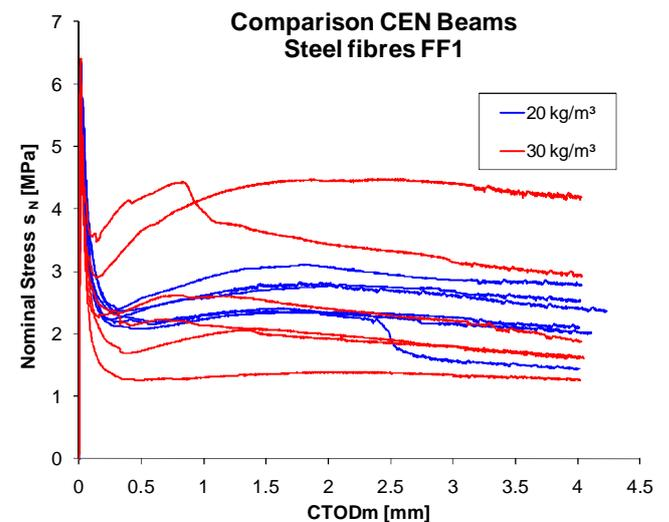
Figure 9. Nominal stress-CTOD of Beam tests according to CEN, for FRC with 20 and 30 kg/m<sup>3</sup>.
