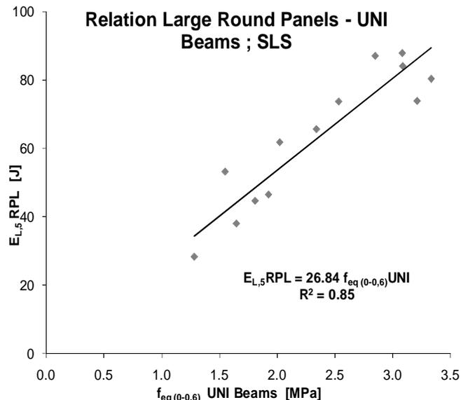
Figure 16. Correlations between energy absorption and equivalent post cracking strength: Classical Large Round Panel tests ASTM vs. Beam Tests UNI, serviceability limit states.
