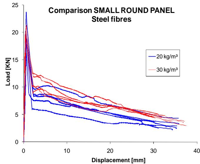
Figure 11. Load-Displacement curve of Small Round Panel Tests, for FRC with 20 and 30 kg/m<sup>3</sup>.
