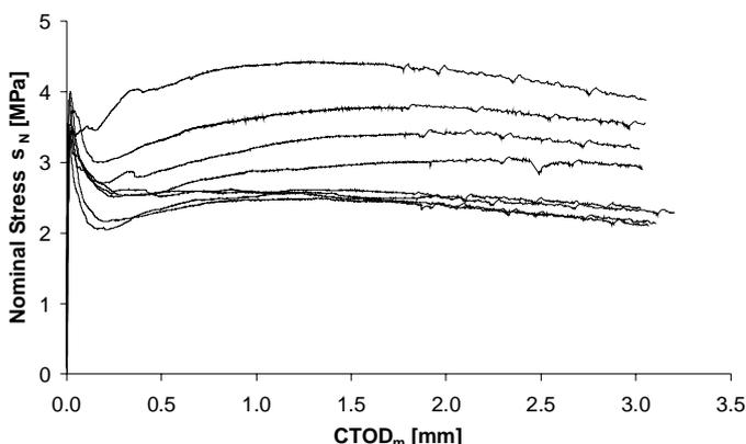
Figure 1. Experimental results from bending tests on notched beams (di Prisco et al. (1), 2004).
