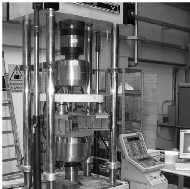
Figure 5. Set up for performing Large Panel tests.
