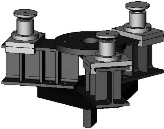
Figure 6. Steel supporting frame for performing Small Panel tests.
