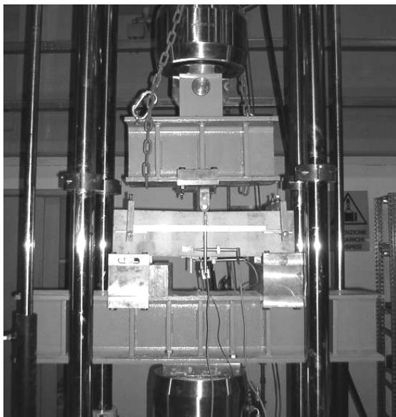
Figure 3. Set up for performing beam tests.
