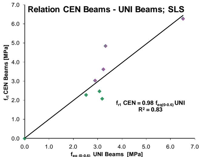
Figure 20. Correlations between residual stress and equivalent post cracking strength: Beam Test CEN vs. Beam Tests UNI, serviceability limit states.
