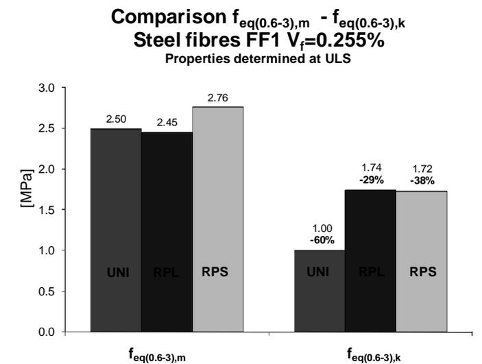
Figure 25. Average vs. characteristic  $f_{eq(0.6-3)}$  using the scatter of different standards: Round Panel tests vs. Beam Tests UNI.
