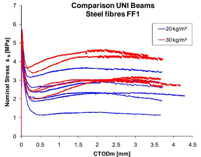
Figure 8. Nominal stress-CTOD of Beam tests according to UNI, for FRC with 20 and 30 kg/m<sup>3</sup>.
