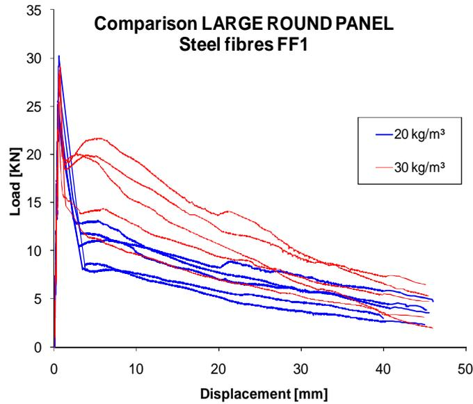
Figure 10. Load-Displacement curve of Large Round Panel Tests according to ASTM, for FRC with 20 and 30 kg/m<sup>3</sup>.
