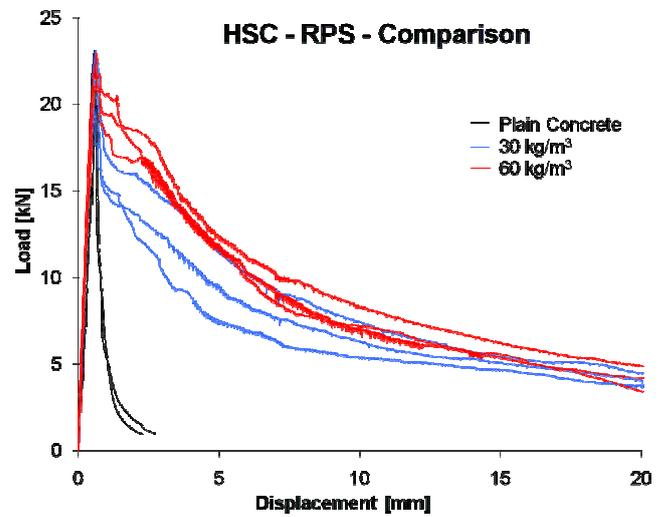
Figure 12. Load-Displacement curve of Small Round Panel Tests, HSC panels, FRC with 30 and 60 kg/m<sup>3</sup>.
