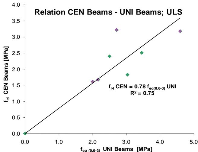
Figure 21. Correlations between residual stress and equivalent post cracking strength: Beam Test CEN vs. Beam Tests UNI, ultimate limit states.
