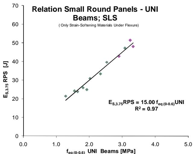
Figure 18. Correlations between energy absorption and equivalent post cracking strength: Small Round Panel tests vs. Beam Tests UNI, serviceability limit states.
