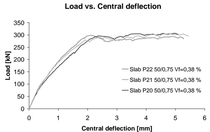
Figure 2. Experimental results from full-scale slabs on grade made of the same FRC as for Figure 1 (di Prisco et al. 2004).
