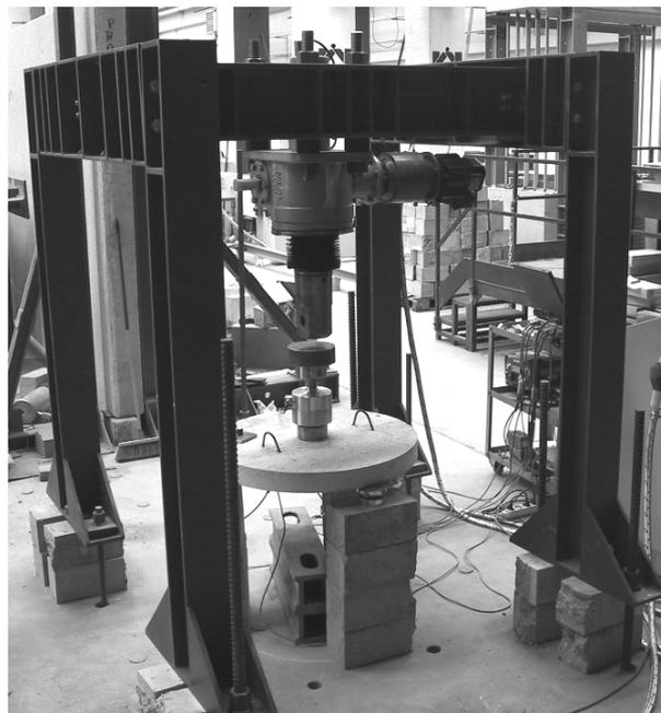
Figure 4. Set up for performing Large Panel tests.
