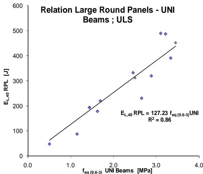
Figure 17. Correlations between energy absorption and equivalent post cracking strength: Classical Large Round Panel tests ASTM vs. Beam Tests UNI, ultimate limit states.
