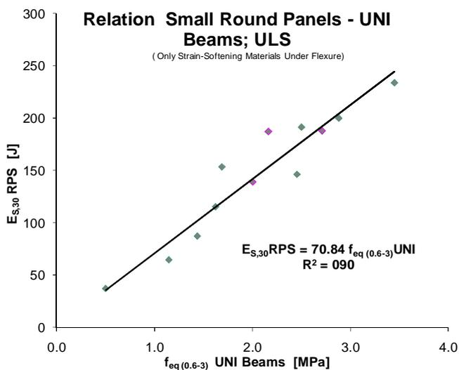
Figure 19. Correlations between energy absorption and equivalent post cracking strength: Small Round Panel tests vs. Beam Tests UNI, ultimate limit states.
