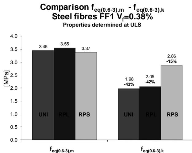
Figure 26. Average vs. characteristic  $f_{eq(0.6-3)}$  using the scatter of different standards: Round Panel tests vs. Beam Tests UNI.
