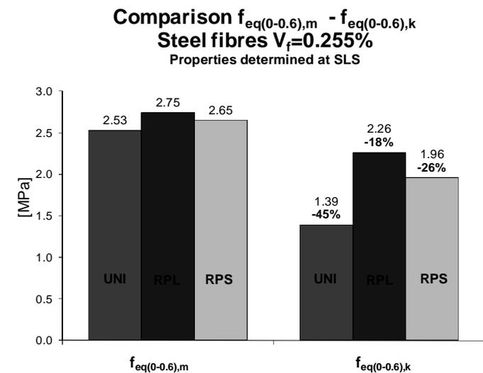
Figure 23. Average vs. characteristic  $f_{eq(0-0.6)}$  using the scatter of different standards: Round Panel tests vs. Beam Tests UNI.
