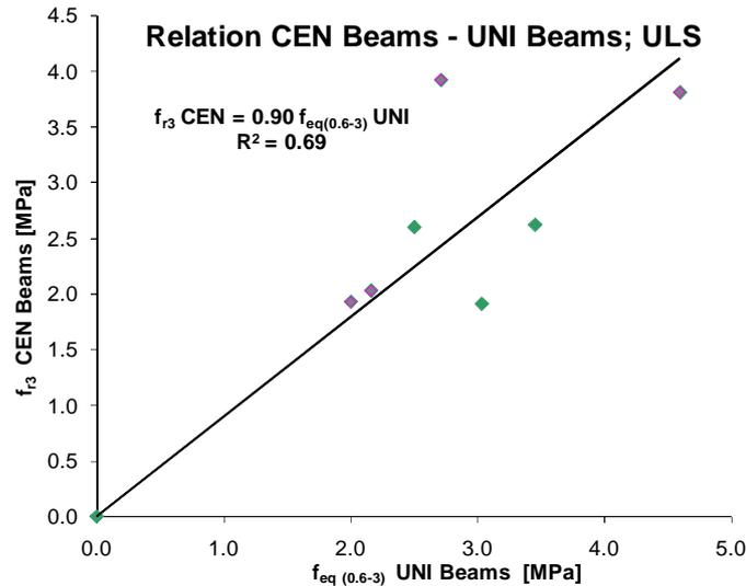
Figure 22. Correlations between residual stress and equivalent post cracking strength: Beam Test CEN vs. Beam Tests UNI, ultimate limit states.
