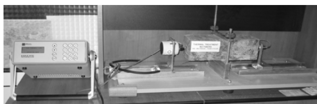
Figure 3. Resonant-frequency testing apparatus.
