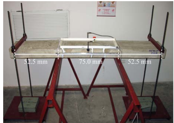
Figure 6. Experimental setup used for the long-term test. The container used to keep the saline solution can be seen in the centre of the picture.
