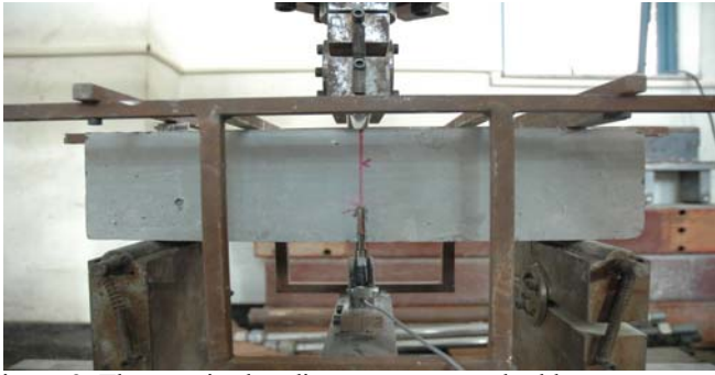
Figure 3. Three-point bending test on a notched beam.
