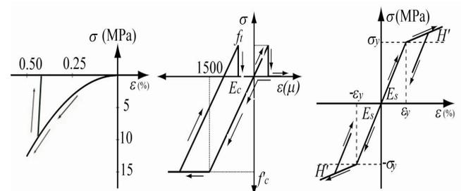
(a) Paving Sand (b) Concrete (c) Reinforced Concrete
