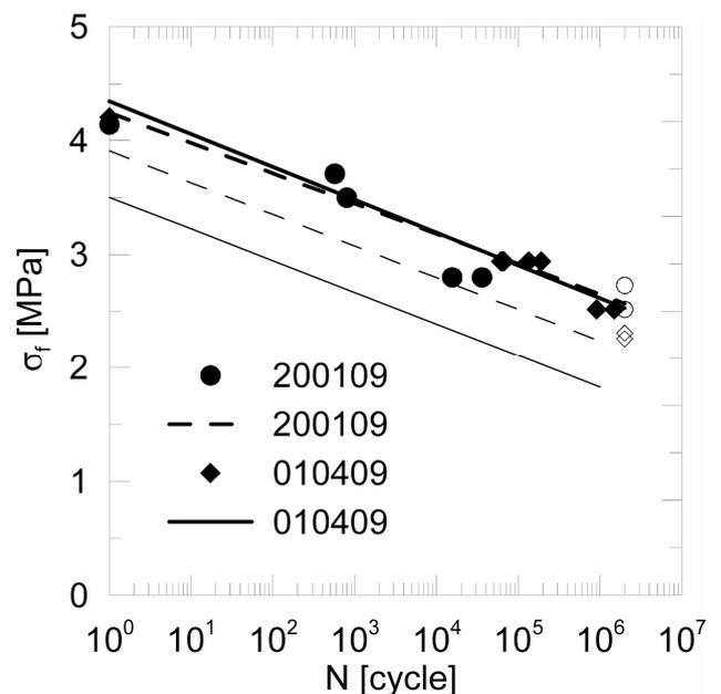
Figure 2.  $\sigma_f$ - $N$  diagrams for 200109 and 010409 materials (black symbol: broken specimen; white symbol: unbroken specimen).
