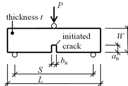
Figure 1. Schematic of three-point bend (3PB) specimen geometry.
