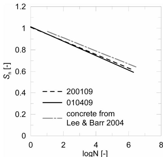
Figure 5. Comparison between  $S_n$ - $\log N$  diagrams for 200109, 010409 materials and literature data Lee & Barr (2004).
