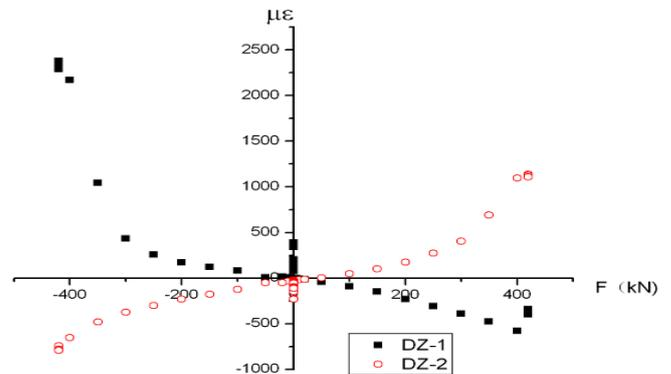
Figure 5-a. side column steel strain.
