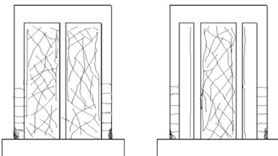
Figure 4. distribution of wall cracks.
