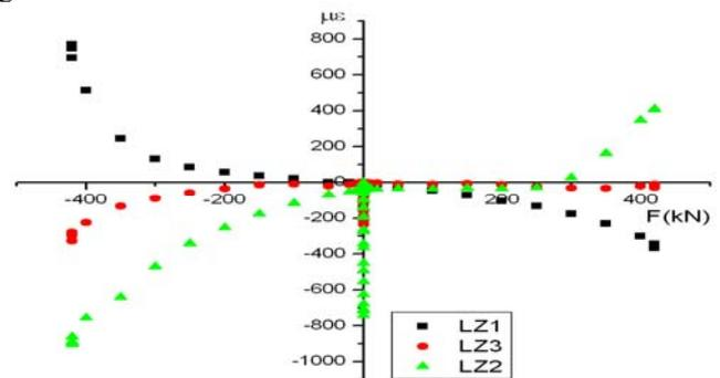
Figure 5-b. rib column steel strain.
