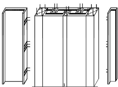
Figure 1. concrete composite bearing wall.
