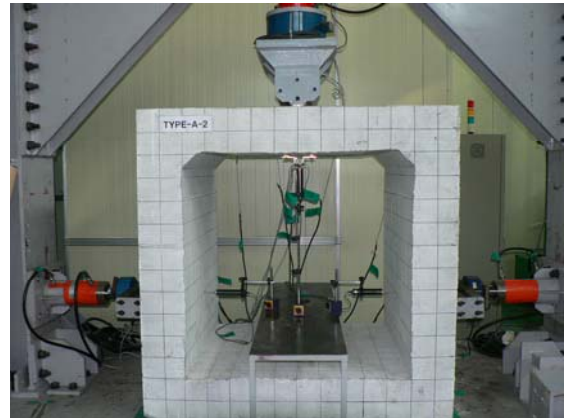
Photo 1. Set up of specimen in the 3-axes loading system.
