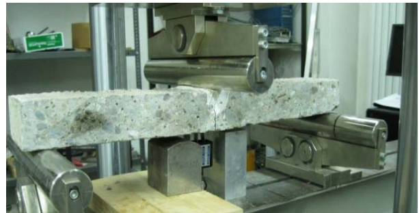
Figure 2: 3-point bending test set-up
