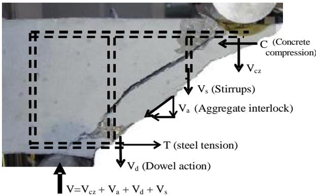
**Figure 1:** Mechanism of shear forces in a beam with transverse reinforcement
