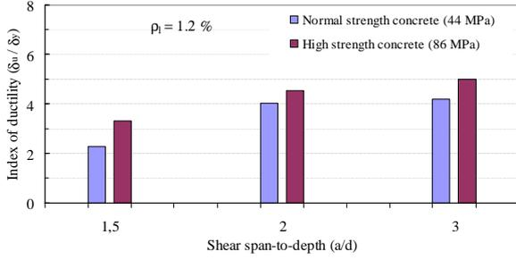
**Figure 8:** Effect of the shear span-to-depth ratio on the ductility factor
