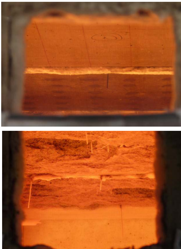
Figure 5: Inside the furnace, view to the bottom side of the specimen at the beginning (top) and during (bottom) the experiment without PP-fibres.
