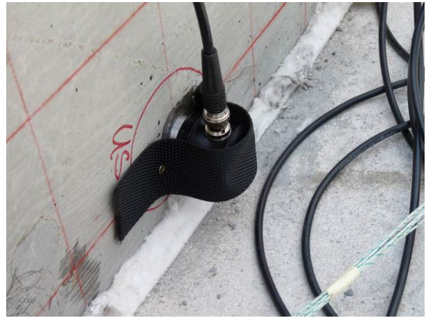
Figure 8: Coupling of Ultrasonic emitter and receiver.
