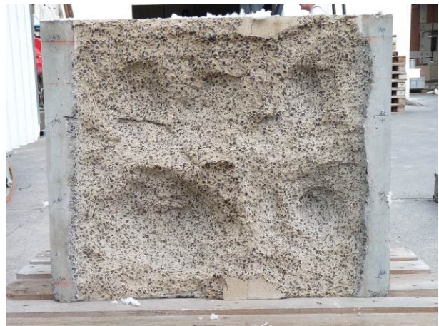
Figure 6: Specimen with 1 kg PP fibers per m^3 concrete after the experiment (top), specimen without PP fibers showing damage due to spalling (bottom).
