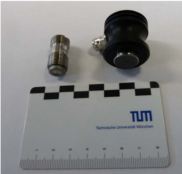
Figure 4: Acoustic emission sensors used on two specimen on top of the furnace.
