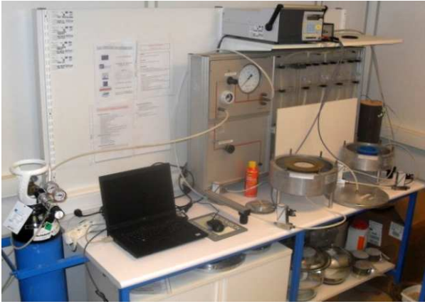
Figure 1: General view of gas permeameter (The CEMBUREAU), (GeM Laboratory - UIT of Saint-Nazaire (France))
