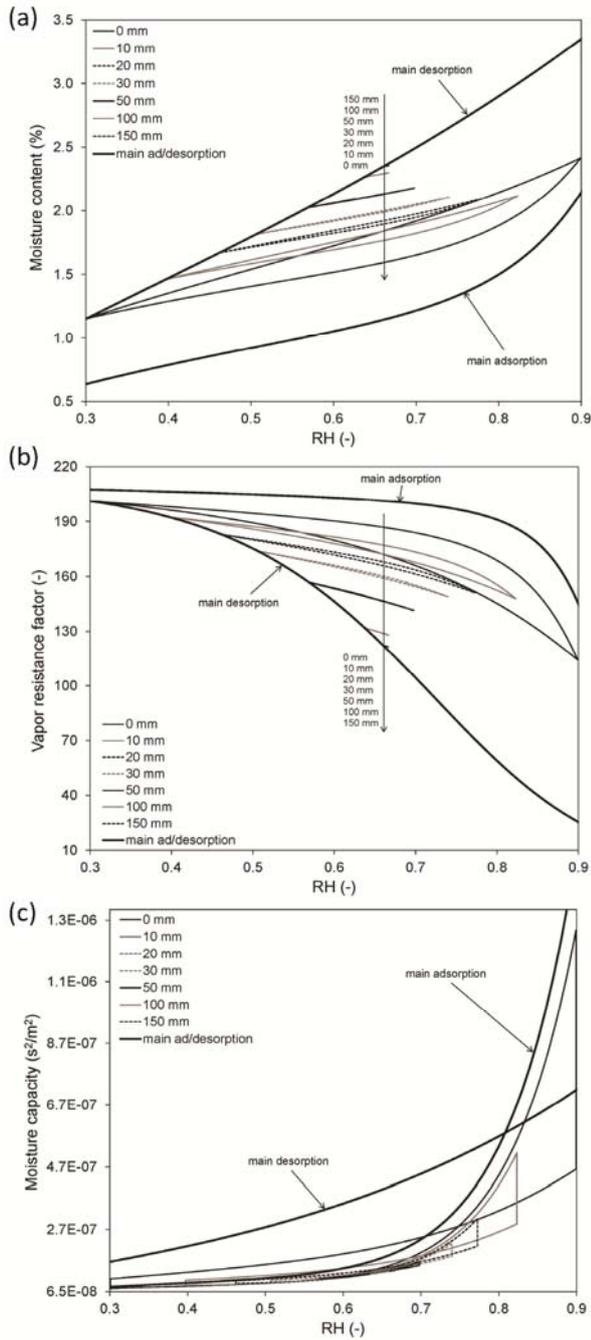
**Figure 5.** Moisture content, vapor resistance factor and moisture capacity in function of relative humidity in a 30 cm thick concrete sample during the last year of 40 years exposure. The sample is initially in a ‘wet state’ (90% RH) and subjected to relative humidity fluctuations between 90 and 30% RH with a 1-year period.
