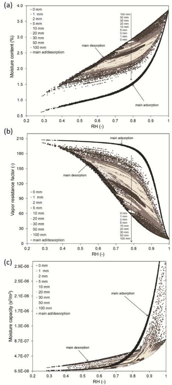
**Figure 6.** Moisture content, vapor resistance factor and moisture capacity in function of relative humidity in a 30 cm thick concrete sample during the last year of 40 years exposure. The sample is initially in a ‘wet state’ (91% RH) and subjected to the outdoor climate of Essen, Germany.
