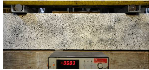
Figure 5: Image analysis disposal with feedback of the load in the foreground
