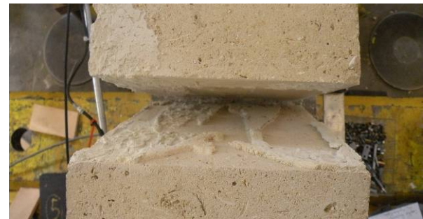
Figure 8: Irregularity of the mortar for the stone assemblage
