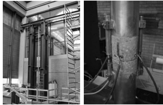
Figure 9: SHB test set-up and instrumented specimen
