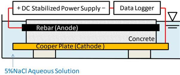
Figure 7 : Corrosion test of the electrolytic corrosion.
