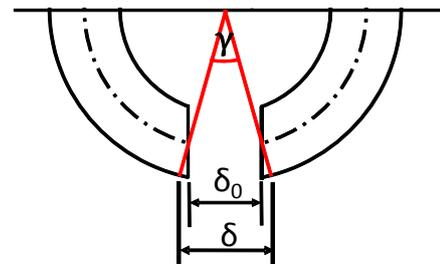
Figure 5 : Corrosion crack and crack angle.
