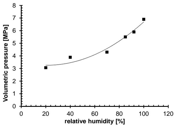
Figure 9: Variation of volumetric pressure at failure with RH.
