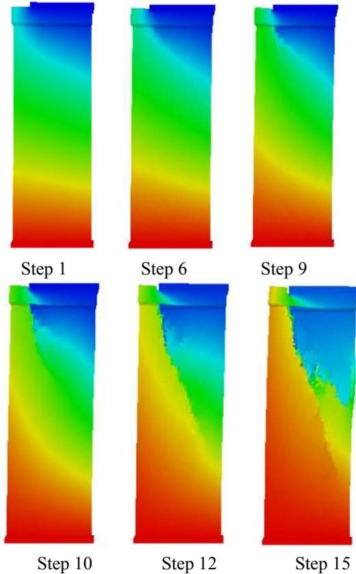
Figure 8: Failure process of  $D_1/D= 3/4$ .
