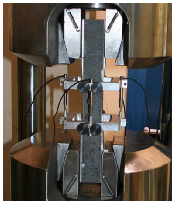
Figure 7 Direct tension test: testing of a 432 mm long specimen
