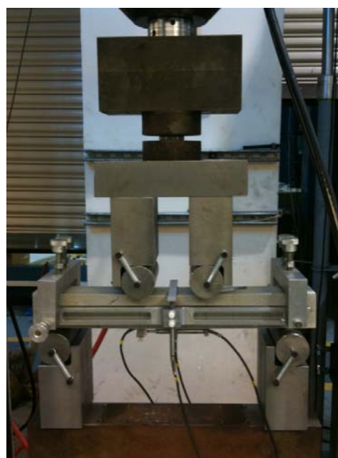
Figure 6 Prism flexural test setup
