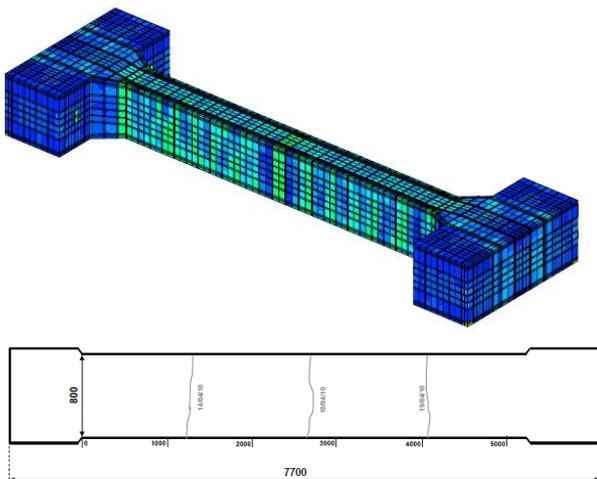
**Figure 11:** Comparison of crack pattern with numerical results
