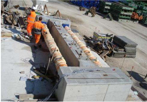
**Figure 6:** Restrained shrinkage specimen
