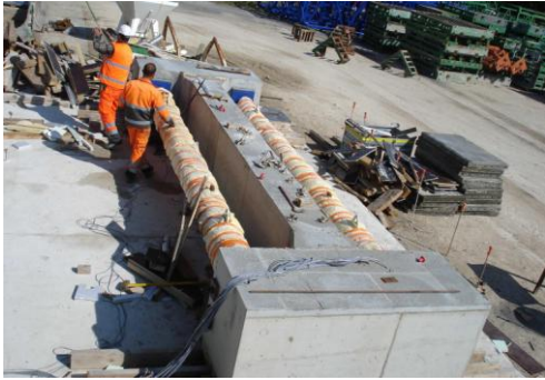
Figure 6: Restrained shrinkage specimen
