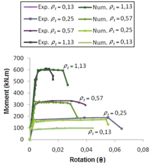
Beam Dimensions: L = 6000 mm x h = 600 mm x b = 300 mm
