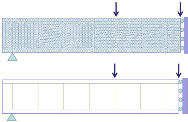
**Figure 3:** Finite element mesh, geometric distribution of the steel bars and stirrups, and boundary conditions of the beam
