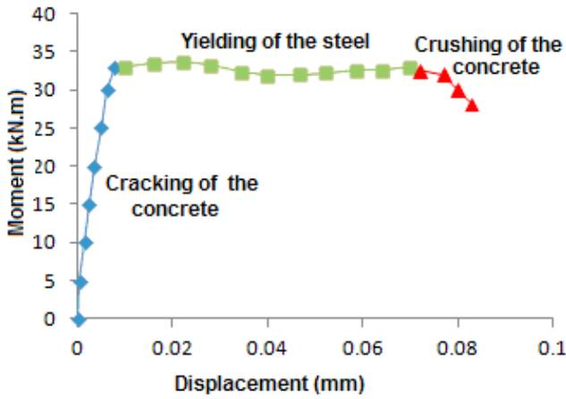
Figure 7: Phases of the structural behavior (B1,  $\rho_t = 1,71$ )
