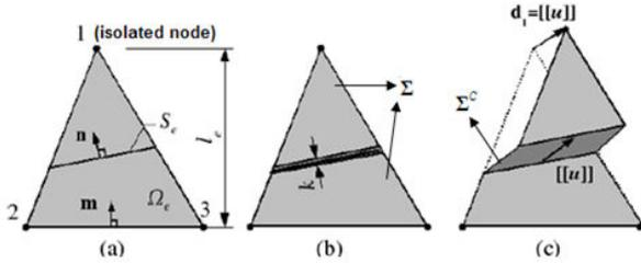
Figure 1: Element with embedded localization band [2]
