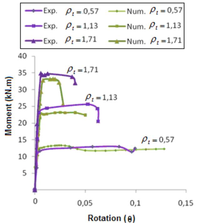
**Figure 5:** Moment vs. rotation curve, comparing the structural responses obtained numerically and experimentally
