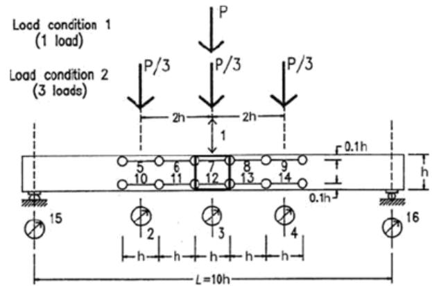
Figure 2: Geometric model of the beam [3]
