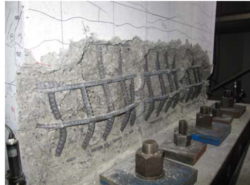
Figure 5: Damaged part after initial loading.
