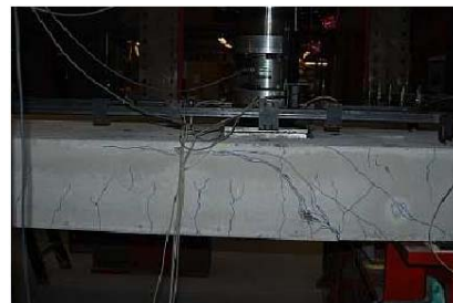
Figure 5: Experimental crack pattern of S4T1 slab on the front face.
