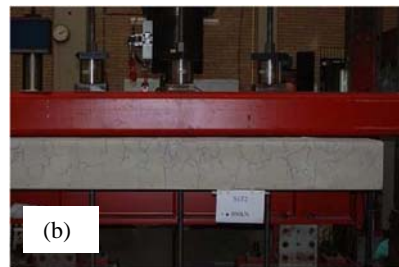
Figure 4: Experimental crack pattern of S1T2 slab (a) at bottom side, (b) on the front face.
