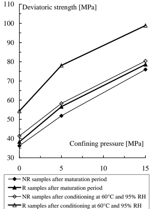
**Figure 2:** Deviatoric strength versus confining pressure for NR mortar and R mortar after maturation period and after conditioning at 60°C and 95% RH.
