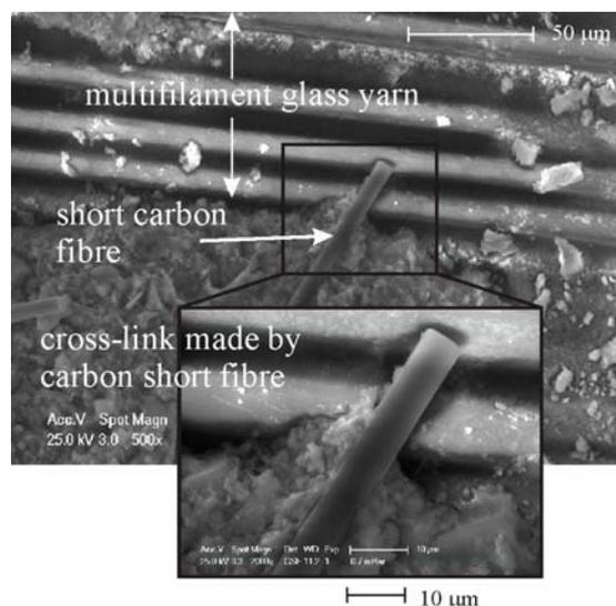
**Figure 12:** “Cross-link” between multifilament-yarn and matrix caused by a short carbon fibre.
