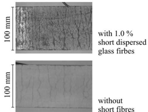
Figure 7: Effect of dispersed short AR glass fibres on the cracks pattern on specimen's surface.
