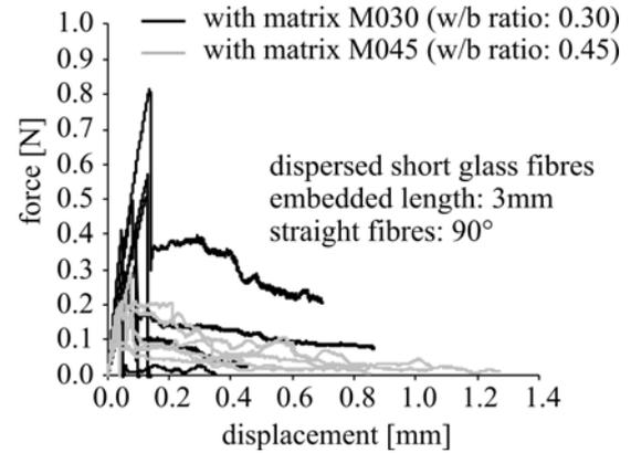
**Figure 9:** Force-displacement curves obtained from the single dispersed glass fibre pullout tests with matrix M030 and matrix M045.
