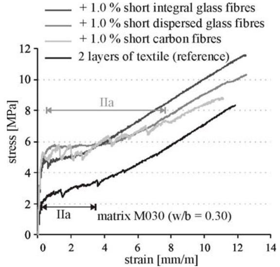
Figure 6: Effect of addition of short dispersed glass, integral glass and carbon fibres on the characteristic stress-strain behaviour of TRC plates subjected to tensile loading.
