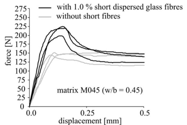
**Figure 8:** Results of multifilament-yarn pullout tests with the matrix M045 with and without the addition of 1.0 % short dispersed glass fibres.
