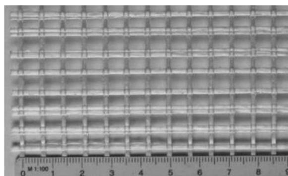
**Figure 1:** Textile reinforcement (AR-glass).
