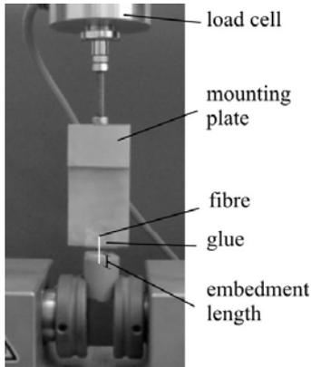
Figure 5: Testing device for single-fibre pullout tests.
