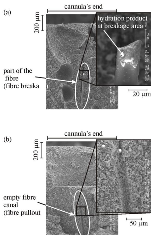
**Figure 13:** ESEM images on single-fibre pullout specimen with matrix a) M030 and b) M045.
