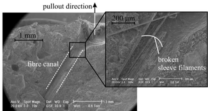
**Figure 14:** Three characteristic curves obtained from the single-fibre pullout tests performed on inclined integral fibres and the corresponding ESEM images: a) completely fixed fibre, b) easily pulled-out fibre, and c) typical fibre pullout response.
