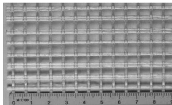
**Figure 1:** Textile reinforcement (AR-glass).
