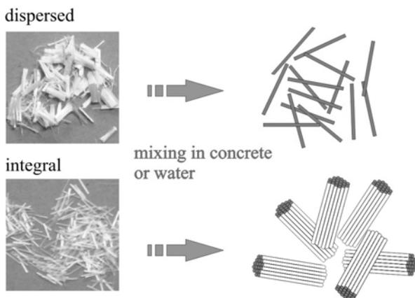
**Figure 2:** Graphic presentation of the condition of fibres used in this investigation when mixed with water or concrete.
