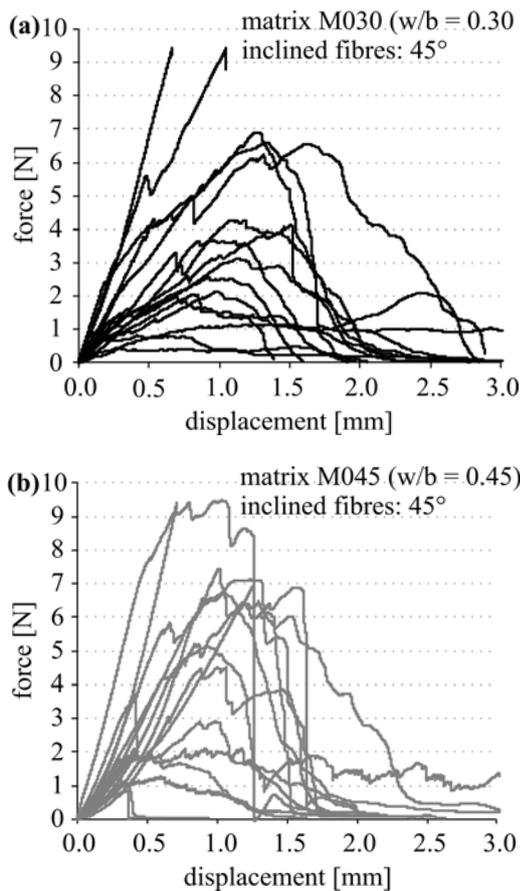
**Figure 11:** Force-displacement curves obtained from the single inclined integral glass fibre pullout tests with the matrix a) M030 and b) M045.
