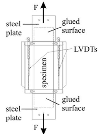
**Figure 3:** Schematic view of the test setup used in uniaxial tension tests.
