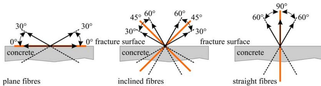
**Figure 10:** Classification of the fibre orientations in respect of the fracture surface.
