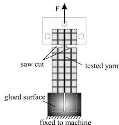
**Figure 4:** Schematic view of test setup used for multifilament-yarn pullout tests.
